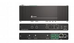
SWT3-21-H is an intelligent 2x1 automatic switcher for 4K60 4:4:4 HDMI video signals, with plug and play user experience such as priority or last-connected auto-switching based on active video signal detection, and easy remote IP-driven management and control
